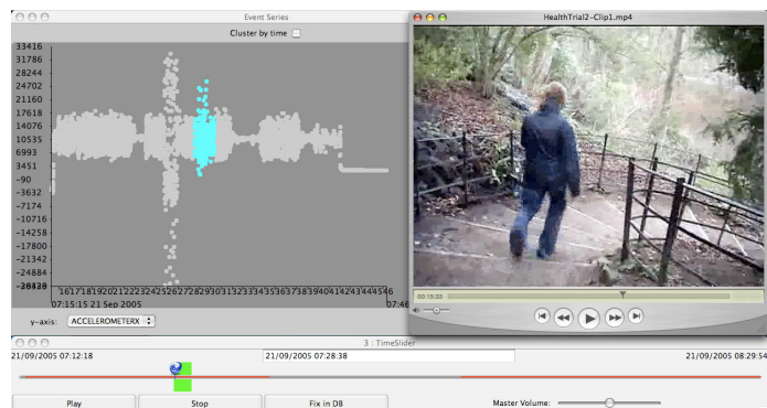
FIGURE 1: Replayer analysing heterogeneous data. A period of the graphed accelerometer logs (left) has been selected, highlighting in green the corresponding time in the video timeline (bottom) and jumping the video to the appropriate section.
